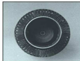
Material deposits on used ion laser bore
